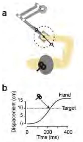
Figure 4.1 a. Experimental set-up. Subjects were seated in front the robot and were asked to hold the handle and ‘shoot’ through a 10 cm distant target in 230ms. b. TMS was delivered when the hand crossed the target during force-field trials.
